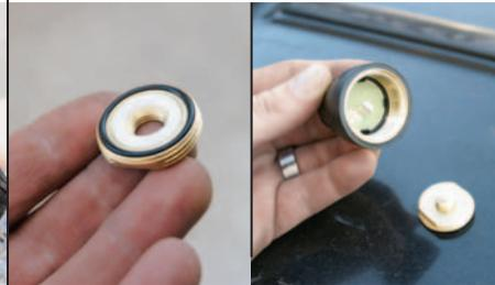
The PCI antenna features a well-designed base with a double nylon-and-rubber O-ring seal. The antenna mount then threads atop the base to complete the connection.
