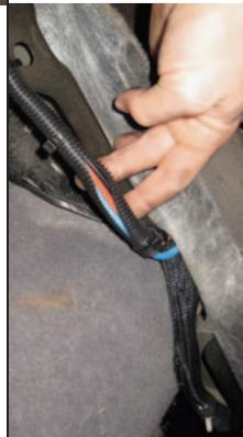
For the microphone, we bought a 5-foot length of network cable and routed it to the center console where we'll install a female Cat 5 connector so we can plug in the mic only when the radio is in use. Once the cables were in place, we tied them up with some wire loom and zip ties.
