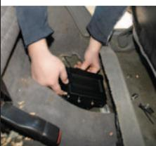
With the mounting holes having been drilled, we placed the radio in the provided cradle mount and secured it in place.
