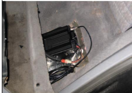
The antenna cable was then routed forward and connected to the radio. With the rear mounting of the head unit, we'll also likely install a small external speaker in the console, but for the time being the speaker in the head unit is sufficiently loud.
