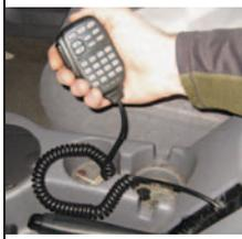
With the additional length of Cat 5 network cable routed to the center console, we attached the mic to a female-to-female adapter and routed it through the emergency-brake lever opening. We'll eventually install a Cat 5 plug in the console to the right of the opening so the mic can simply be plugged in. Check out the *4WD&SU* blog at [www.4wdandsportutility.com](http://www.4wdandsportutility.com) to see the finished product.
