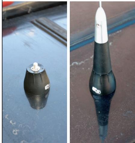
When the radio isn't in use, we can keep the antenna in the cab and then simply thread it onto the base upon use. We'll likely put a rubber cap over the threads of the base so the threads will stay clean.
