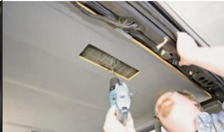
We decided to mount the antenna above the rear dome light since we could hide the cable under the rear overhead speaker bar (not shown). We stepped up drill-bit sizes until a 3/8-inch hole could be cleanly drilled.
