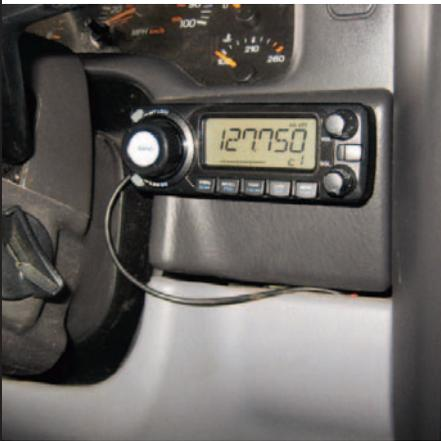
With the separation cable routed to the right of the steering wheel, we attached it to the detachable radio face and used Velcro strips to secure it in place. Icom offers a radio face mount, but we had the Velcro handy and it seems to hold it securely.
