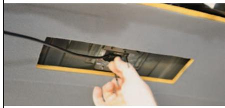
The area of the roof above the dome light is double-sheared, so it was necessary to cut out a portion of the mount. Once removed, the antenna easily passed through the newly drilled hole.
