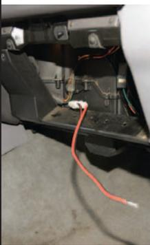
Due to the under-the-rear-seat mounting, the provided fused power-supply cables only reached to behind the glovebox. We added short lengths to each to reach the battery, passing them through a firewall grommet below the passenger-side hood hinge.
