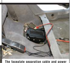
supply cables were attached to the radio and routed under the carpet forward to the center
